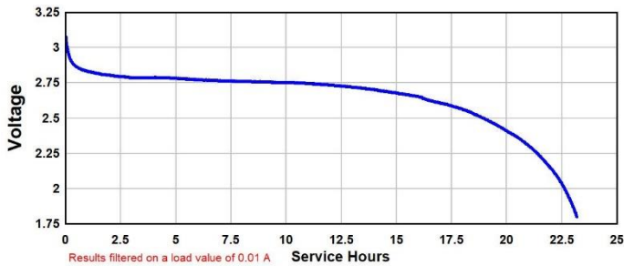
IEC Key Fob Performance 10 mA 5s/m to 1.8V
