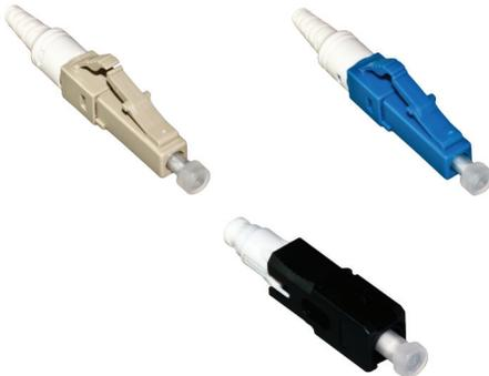
The XP Fit Plus Connectors are a pre-polished, pre-assembled, non-epoxy fibre connector compatible with standard SC and LC connectors. Without polishing or adhesives, the XP Fit Plus makes terminating faster and easier, with a typical connection time of less than two minutes.
