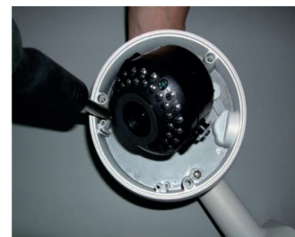
7. Set dome camera body onto cap body with 3pcs of M4xL18 screws.
